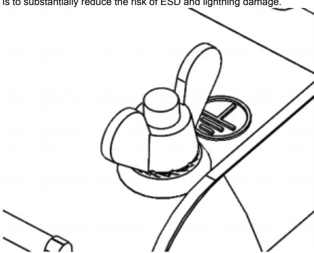
The device includes a grounding connection (marked ).
